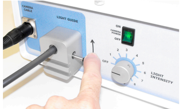
LIGHT CABLE CONNECTION
